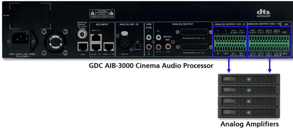
Figure 9: AIB-3000 to Analog Amplifiers
